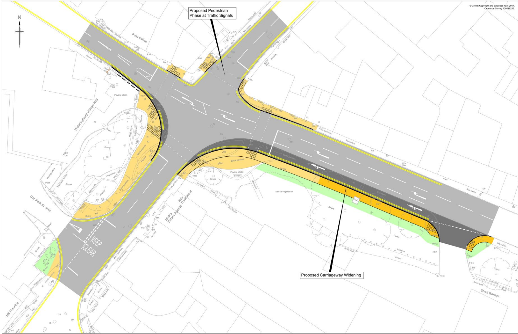
A26 TONBRIDGE ROAD/BOW ROAD/RED HILL, WATERINGBURY PROPOSED MODIFICATION TO EXISTING JUNCTION - OPTION B
